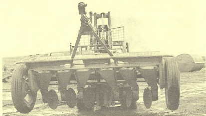
Figure 25. Proper balance of the drill on forklift is important
